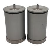
The ignition and burning process is contained within a chamber so that the energy released can be measured in the form of heat. The Vessel has temperature sensors built into it, so that the temperature rise can be measured.
